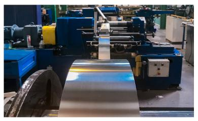
Low Width Thickness Ratio 3:1 unique to the industry (normal minimum is 8:1)
